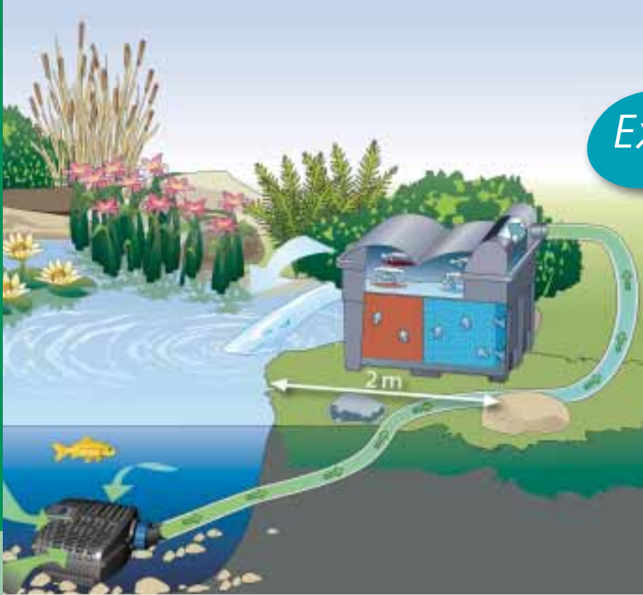
Schematic diagram: BioSmart Set components in function
